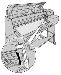
**5** Hold the jammed sheet by the left and right edges and pull it toward you, then cut it where the printing ends or where it is wrinkled.
